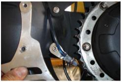
Once fitted, <u>fill and prime the system</u> and set the adjuster knob to 'prime'. Start the engine and turn the adjuster knob until a flow of between 1 and 2 drops per minute is achieved. Check the condition of your chain after a ride, and then adjust as required.
